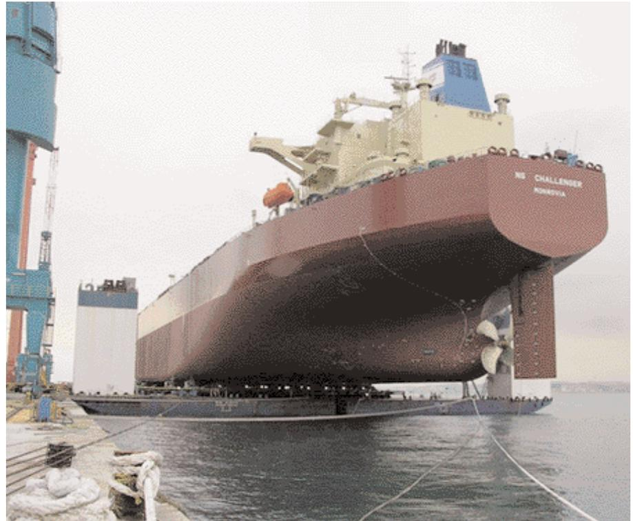
**The Air Pad Sliding system (APS) developed by Hebetec uses jacks and air pads to launch boats that are built on dry docks.**
