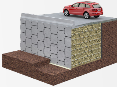
Reinforced Earth walls
