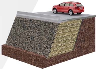
Reinforced Earth slopes
